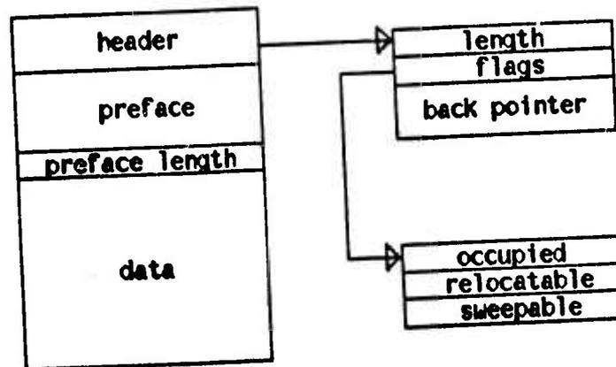
*Structure of the FLAGS field in a BLOCK HEADER*
