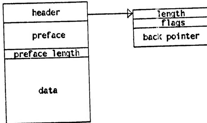
*Structure of a BLOCK HEADER*
