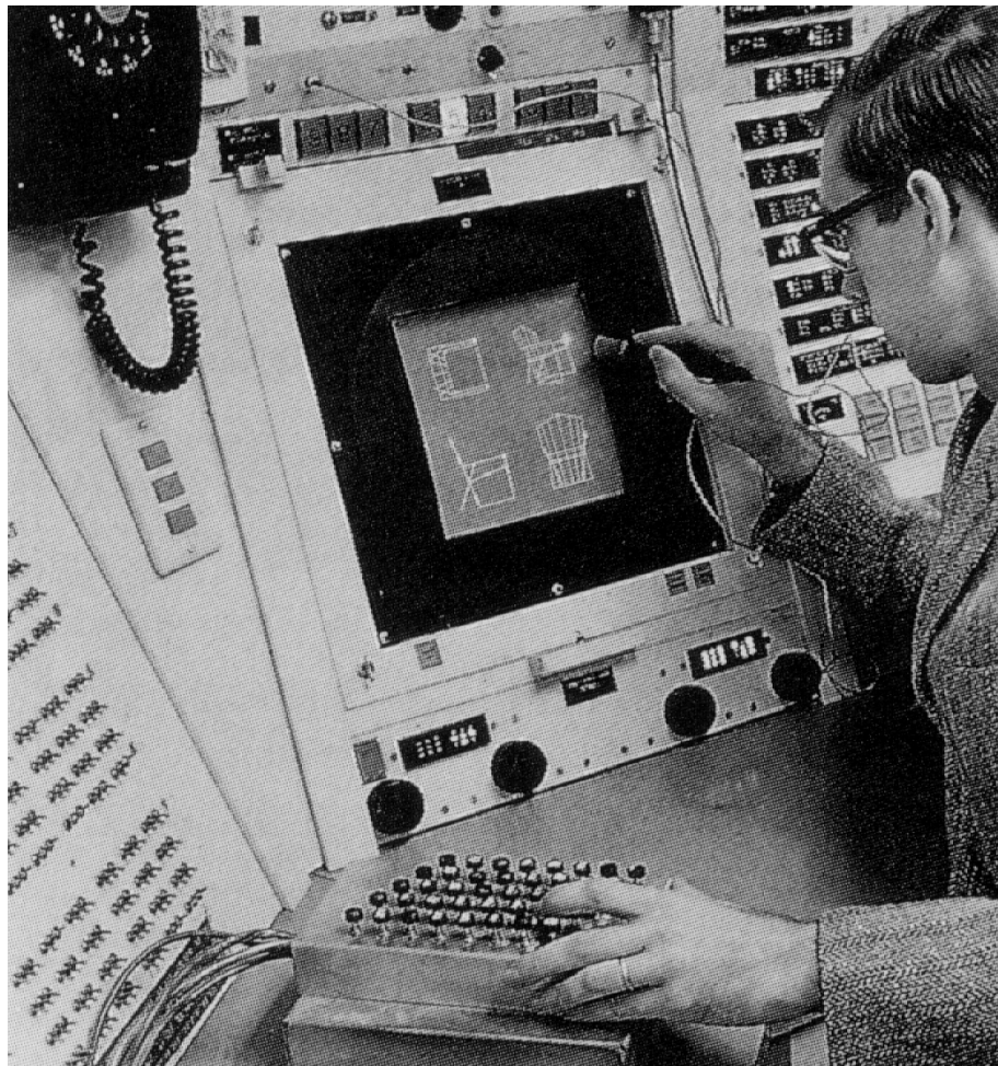
Fig. 3.1 Ivan Sutherland's Sketchpad console, 1962. Sketchpad is operated with a light pen and a command button box (under left hand). The four black knobs below the screen control position and scale of the picture.
