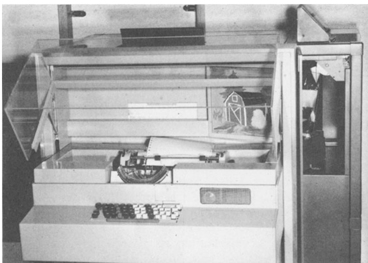
Figure 3. E.R.E. ( The Edison Responsive Environment ) or "Talking Typewriter"
