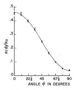
**Figure 19.** Coincidence rate vs. angle  $\phi$  between the polarizers, divided by the rate with both polarizers removed. The solid line is the prediction by quantum mechanics, calculated using the measured efficiencies of the polarizers and solid angles of the experiment.
