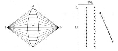
**Figure 9.** Situation identical to Figure 8 but with a piece of glass added. The shape of the glass is such that all paths from the source S reach P in phase. The result is an *enormous* increase in the amplitude reaching P. (From Fig. 36 in Feynman's **QED**).
