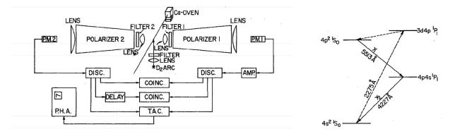
**Figure 16.** Left: Schematic of the polarization-correlation experiment. Right: Energy levels of the Ca atoms used in this experiment. From Freedman and Clauser 1972 [6].
