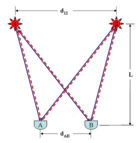
**Figure 14.** Schematic diagram of the Hanbury–Brown–Twiss effect, with excited atoms 1 and 2 in distant separated sources simultaneously exciting ground state atoms *A* and *B* in two separated detectors.
