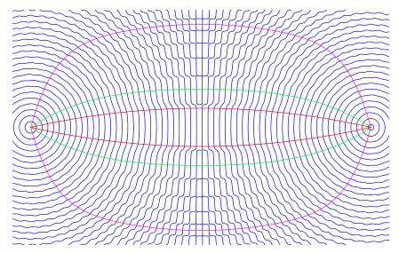
**Figure 13.** The zero crossings of the handshake vector potential at t = 0. Paths near the axis (between the two red lines) are responsible for the conventional 1/r dependence of the potential. Paths shown through high-amplitude regions have an even number of zero crossings, and thus the potentials traversing these paths all arrive in phase, thus adding to the central potential.
