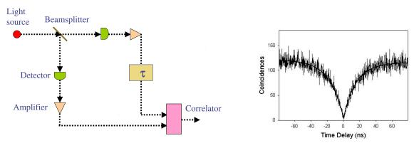
Figure 15. Left: Schematic of the photon-splitting experiment. Right: Plot of the number of coincidences vs. time delay between the arriving pulses. The source on average generates a photon per  $\approx$ 12 nsec. The finite number counted at zero delay is consistent with the accidental presence of two excited atoms.
