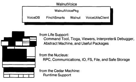
Fig. 8. The WalnutVoice component depends directly on four application components and fifteen Cedar interfaces from the Life Support, Nucleus, and Cedar Machine layers. The fifteen system components are shown as dark areas on the small version of Figure 2 below.
