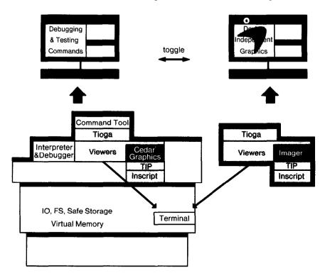
Fig. 6. The replacement of the Cedar Graphics package by the new Imager package required binding the Imager and its clients together to avoid interface mismatches.
