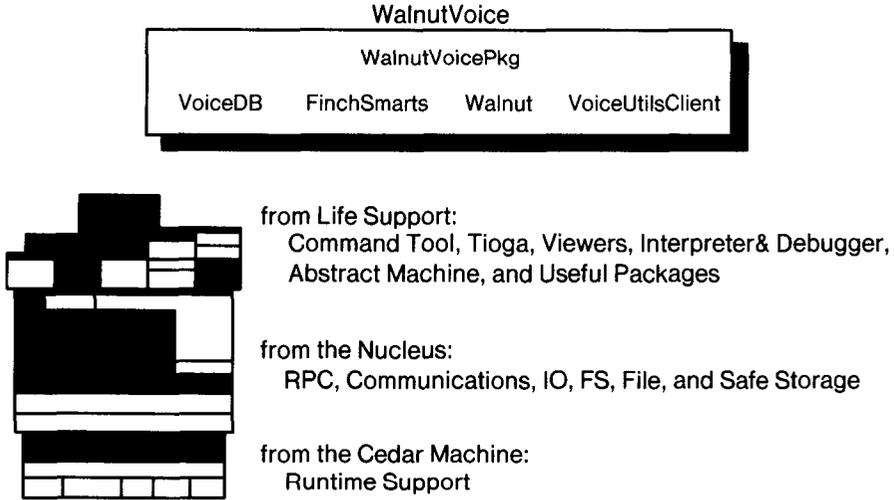
Fig. 8. The WalnutVoice component depends directly on four application components and fifteen Cedar interfaces from the Life Support, Nucleus, and Cedar Machine layers. The fifteen system components are shown as dark areas on the small version of Figure 2 below.
