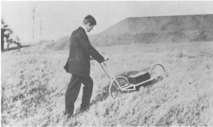
FIG. 10.—Bush testing the Profile Tracer near the reservoir at Tufts College. (Courtesy of the MIT Museum and Charles Eames, Venice, California. The photo is from Bush's 1913 master's thesis, "An Automatic Instrument for Recording Terrestrial Profiles.")
