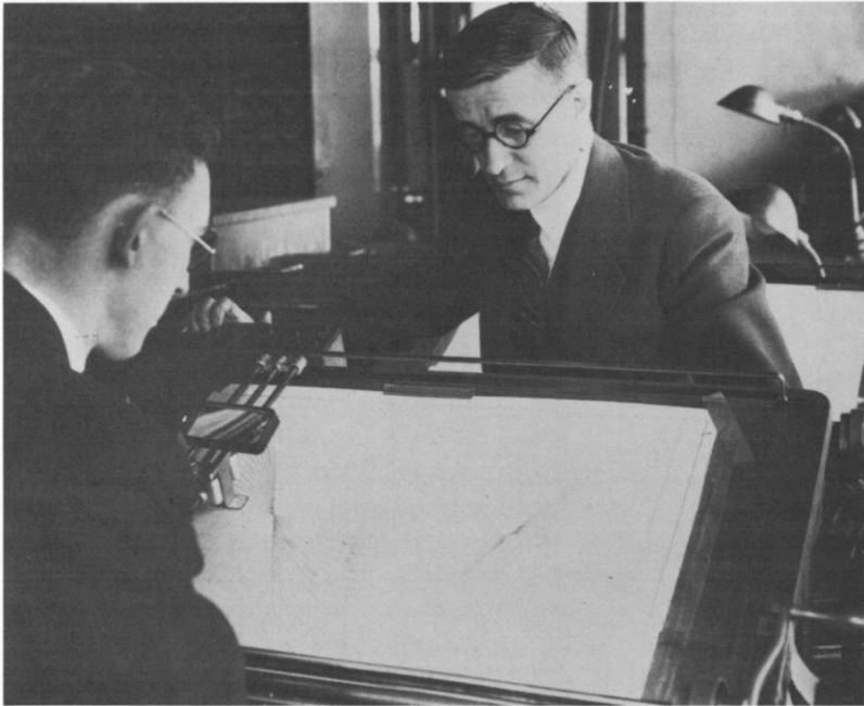
FIG. 7.—Bush and Caldwell standing at the output board of the Differential Analyzer inspecting a family of curves produced during the solution of an equation. (Courtesy of the MIT Museum.)
