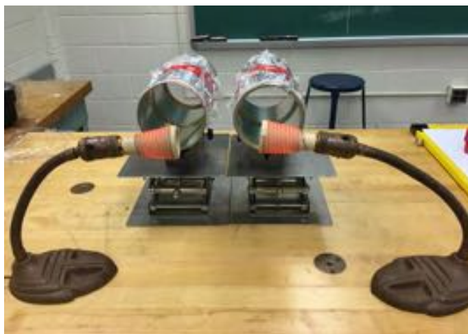
Figure 6.2: Setup. After irradiation from the two heat lamps ( foreground ), the two cans were viewed by an infrared camera placed on the far side (near the chalkboard). Not shown : For the trial shown in Fig. 6.3, each cylindrical can was wrapped in a blanket of foam insulation (except for its ends).
