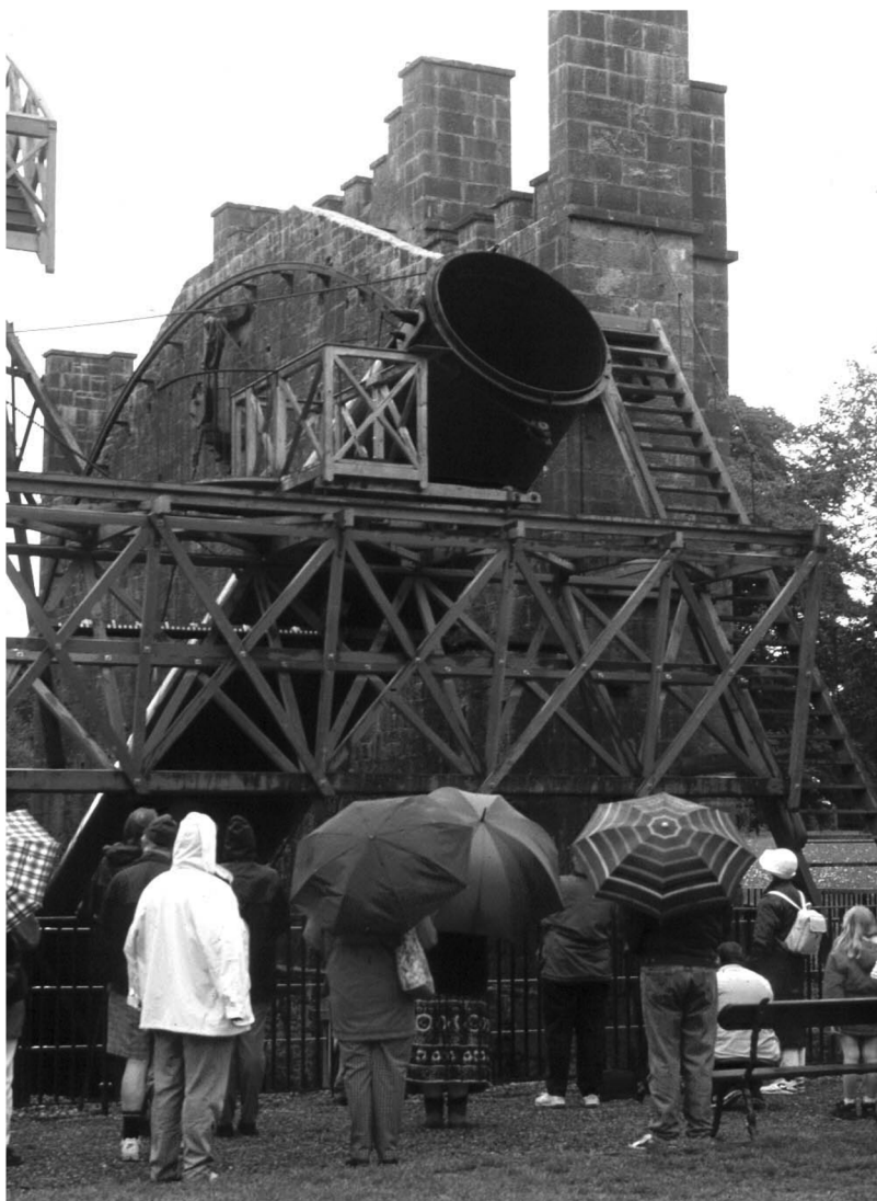
Rosse Telescope. In 1845 William Parsons, the Third Earl of Rosse, put the largest telescope of the nineteenth century into operation on his family estate in Birr in central Ireland. The four-ton, six-ft diameter speculum metal mirror was cast and figured by the Earl (1800-1877), who also designed the telescope. The instrument, with a focal length of about 60 ft, was used for visual observations of nebula, which were then drawn, quite accurately, by hand. The telescope is still in operation, but with a lighter, aluminum mirror that is coated with bronze to give the same reflectivity as the original mirror. Electric motors now move the telescope tube about instead of the five men who originally turned capstans. The picture was taken on a typical, slightly rainy day in September 1999. (Notes and photograph by Thomas B. Greenslade, Jr., Kenyon College)
