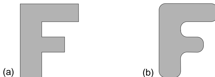
Figure 4.9 Rounding right angles in an F. (a) The unrounded version; (b) After application of our rounding rule. (This figure has been reduced.)
