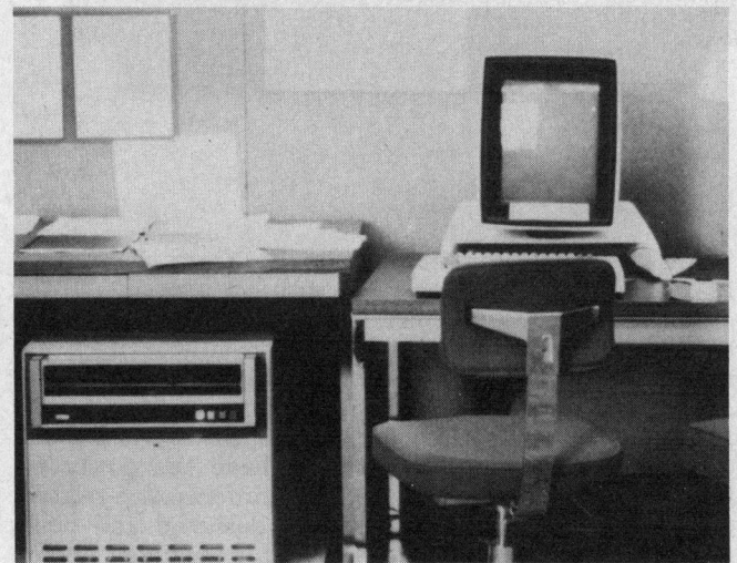
Figure 3. The interim Dynabook system consists of processor, disk drive, display, keyboard, and pointing devices.
