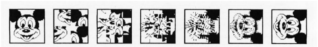
Fig. 11. 90-degree rotations accomplished by masking, shifting, and storing operations, all of which can be implemented with BitBlt. Figure taken from Byte [Ingalls 1981, p.188].
