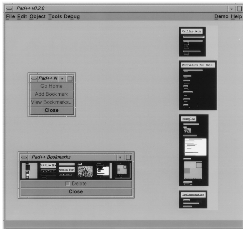
Figure 3. Visual bookmarks let users remember interesting places they have been by showing miniature views of those places. Clicking on one of the views animates the main view to the location
