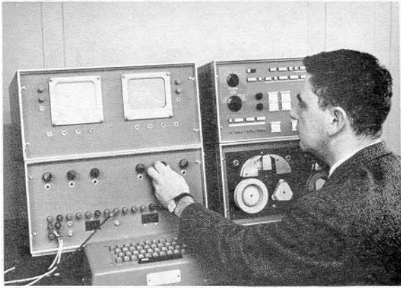
William Simon with an interim version of the LINC. The dual-display module provided both long- and short-persistence phosphor CRTs. Six potentiometer knobs supplied input parameters.
